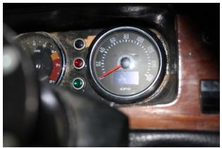
The GPS unit included a high beam indicator and left/right turn signal indicators. The Europa has a blue high beam indicator, and a green turn signal indicator separate from the speedometer. I was able to wire onto these and have them work in the GPA unit along with the original indicators.
